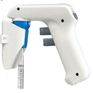
**3 Modes** Bright LEDs indicate 3 operation modes: high, low, & gravity
